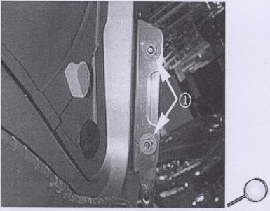
**Important:** Take care to not let the tonneau slide fore-aft when adjusting the position up/down. Loosening only one nut and pivoting on the other nut works well to help control this.
