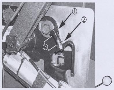
**Note:** When adjusting the jamb nut, do not exceed a distance (3) of 21 mm (0.827 in) from the top of the jamb nut to the bottom of the adjuster stop nut.
